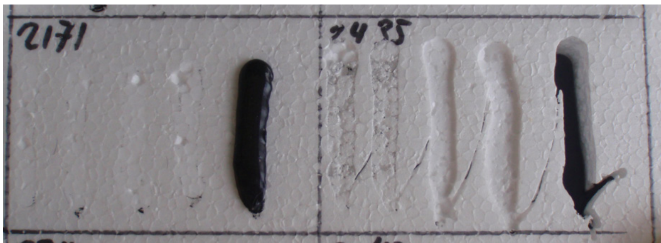
Adhesive compatible with EPS after storage at 80°C
